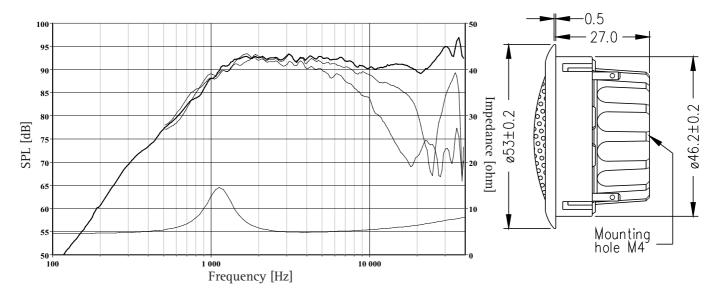
The frequency responses above show measured free field sound pressure in 0, 30, and 60 degrees, mounted in a 0.6m by 0.8m baffle. Input 2.83 Vrms, microphone distance 0.5m, normalized to SPL 1m. The impedance is measured without baffle using a 2V sine signal.
