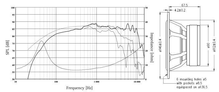
The frequency responses above show measured free field sound pressure in 0, 30, and 60 degrees angle using a 7L closed box. Input 2.83 VRMS, microphone distance 0.5m, normalized to SPL 1m. The dotted line is a calculated response in infinite baffle based on the parameters given for this specific driver. The impedance is measured in free air without baffle using a 2V sine signal.
