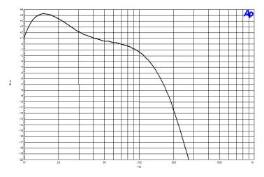
Crossover frequency is set to 120Hz. Bassboost is set at 6dB and 20Hz.
