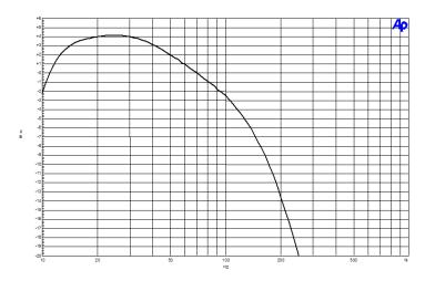
Crossover frequency is set to 120Hz. Bassboost is set at 6dB and 50Hz.
