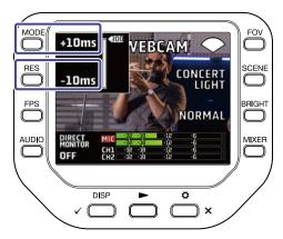
Pressing **+10ms** lengthens the delay time by +10 ms and pressing **-10ms** shortens the delay time by -10 ms.
