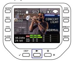
To stop playback and return to the Recording Screen, press  $\overset{\circ}{\bigsqcup}$   $_{\times}$  .
