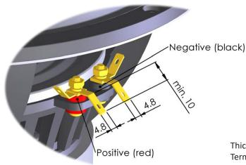
Thickness, both terminals: 0.8 mm Terminal plating: Gold
