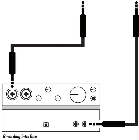
In this example, the TB12 Black is being routed as an insert into a recording device. This is useful for using the TB12 Black as an “analog plug-in” or insert for mix-down. The recording device is feeding the TB12 Black with a balanced 1/4” cable via a line output. Then, the recording device is capturing the TB12 Black via a LINE LEVEL input.
