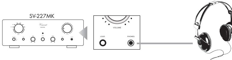
By doing this, the loudspeakers are switched off. All headphones with an impedance of between 32 Ohm and 600 Ohm may be used. Unsuitable headphones with too low impedance may damage the amplifier or produce such unexpectedly loud volume that your hearing may be damaged. The volume (3)(21) should be reduced for safety reasons before a set of phones is connected.
