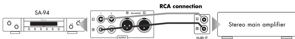
If the main amplifier has an XLR input connector it should be preferred over the RCA input connector. In that case interconnect the XLR connectors named "BALANCED" (9) and the main amplifier input. Please pay attention not to interchange right with left channels. The letters "R" and "L" indicate the correct correlation.
