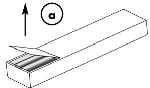
b) If necessary, remove used batteries and insert new ones correctly as shown by the diagram in the battery compartment.
