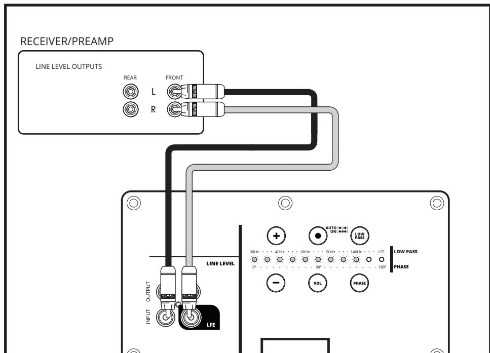
Enable and adjust the on-board low pass filter of the PC-2000 Pro for a smooth blend with the main speakers.
