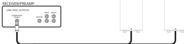
Another option is to use the Left and Right RCA outputs on the PC-2000 Pro to Daisy Chain additional subwoofers. It's important to use the matching output and input terminals. For example, if you are using the RCA inputs, be sure to use the RCA outputs to daisy chain to the next subwoofer.
