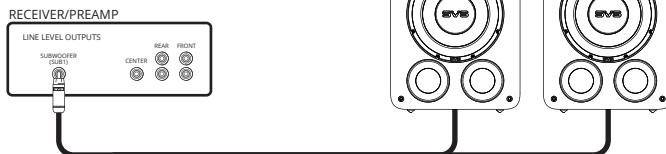
Another option is to use the Left and Right RCA or XLR outputs on the PB-3000 R| Evolution to Daisy Chain additional subwoofers. It's important to use the matching output and input terminals. For example, if you are using the RCA inputs, be sure to use the RCA outputs to daisy chain to the next subwoofer.
