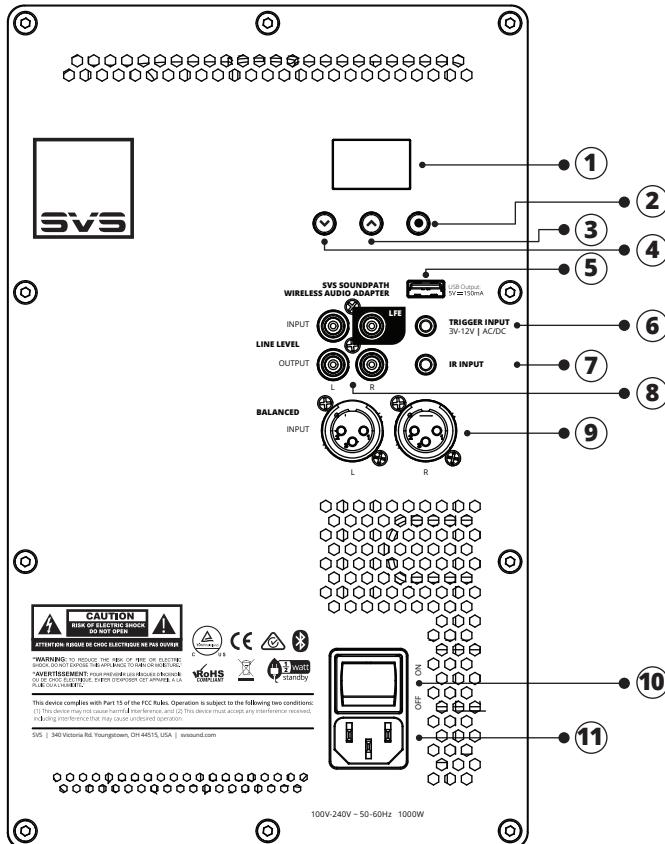
① **OLED Display** - Displays the level for Volume, Low Pass Filter Frequency, Phase, and other settings
