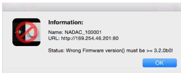
Figure 70. MERGING+NADAC wrong firmware version installed
