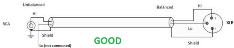
Figure 9. Correct balanced output to unbalanced input connection method.
