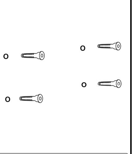
Insert the wall anchors\* to the wall and tap them flush with a hammer.
