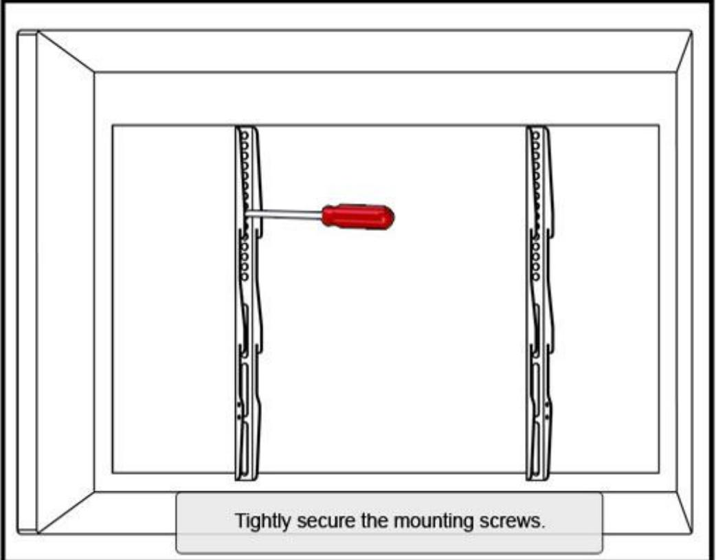
Tightly secure the mounting screws.
