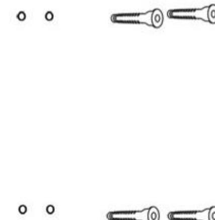
Insert the wall anchors\* to the wall and tap them flush with a hammer.
