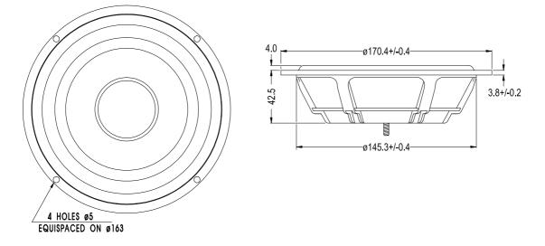
SP17R is a 17cm (6,5") passive radiator intended for use, as an alternative to the vented port in a bass reflex cabinet, together with an active woofer of similar size or smaller.
