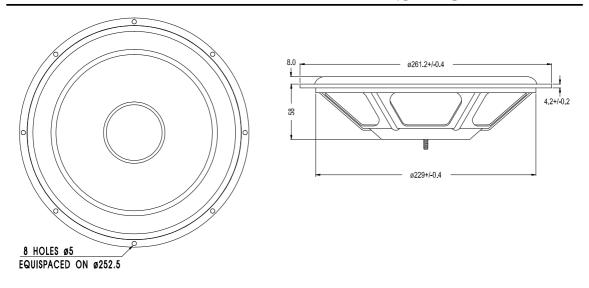
SP25R is a 25cm (10") passive radiator intended for use, as an alternative to the vented port in a bass reflex cabinet, together with an active woofer of similar size or smaller.
