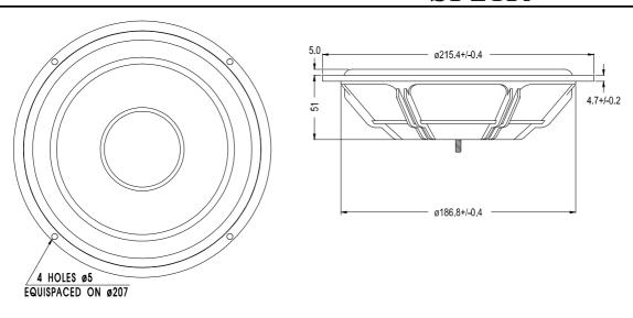
SP21R is a 21cm (8") passive radiator intended for use, as an alternative to the vented port in a bass reflex cabinet, together with an active woofer of similar size or smaller.
