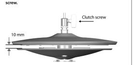
Although the gap can be adjusted to a clearance that makes playing the hi-hat easier, setting too narrow or wide a gap can cause improper function of the unit and prevent the hi-hat from sounding as you intend. Setting the gap to 10 mm provides the most natural feel when playing the VH-14D.
