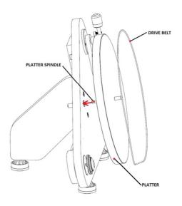
After placing the record on the platter, it is necessary to tighten the screw-able record clamp (6) onto the platter spindle.
