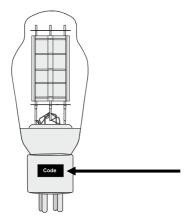
The output tubes you get from Octave are matched with an identical match code Therefore it does not matter where you plug in the tubes: position 1, 2 or 3
