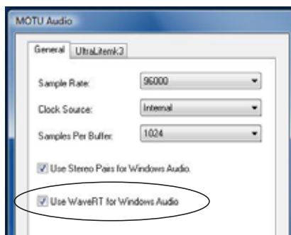
Figure 8-1: The WaveRT option can be enabled in the MOTU Audio Setup console.
