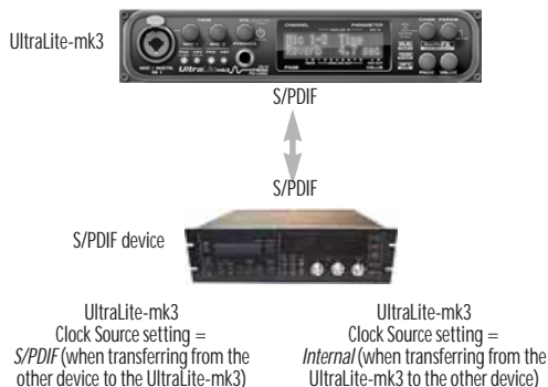
Figure 4-7: The setup for synchronizing a S/PDIF device with the UltraLite-mk3. Sync is achieved via the digital I/O connection itself. In this case, you have to choose S/PDIF as the UltraLite-mk3's clock source when recording from the other device.
