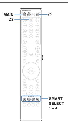
Settings such as the input source, volume level and sound mode can be registered to the SMART SELECT 1 - 4 buttons.
