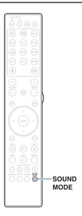
This unit has a selection of sound modes for you to enjoy: a Direct mode that plays audio exactly as it is recorded on the input source, a Stereo mode that adjusts the bass and treble output and a Pure Direct mode that enhances the quality of the audio that is played in Direct mode.
