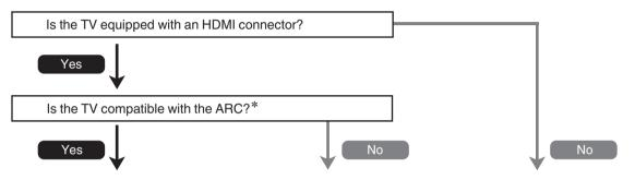
"Connection 1 : TV equipped with an HDMI connector and compatible with the ARC (Audio Return Channel)" ((定) p. 35)
