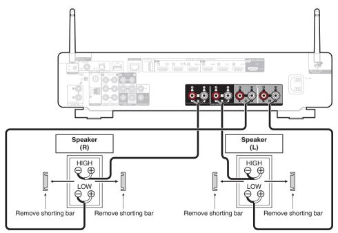
When using bi-wiring connections, set the speaker to "A+B" to output audio from both SPEAKERS A and SPEAKERS B speaker terminals. (27 p. 146)
