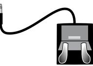
The SW1 (SUSTAIN) and SW2 jacks can be connected to dual switch pedals (2 pedals per jack), allowing up to four switch pedals to be used. Compatible pedals should use a single 1/4 inch tip-ring-sleeve plug.
