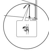
Attach the pedal cord holders **(1)** to the rear panel as shown, then clip the cord into the holders
