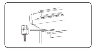
Insert the pedal cord plug to the pedal jack from the rear.
