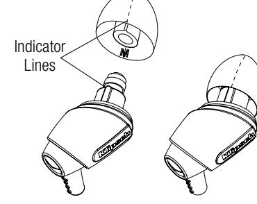
Align indicator lines on the ear tip and headphone nozzle for proper seal.
