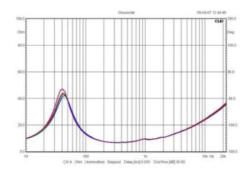
Free air impedance of four JA8008 samples after burn-in. Like most other high-efficiency drivers the JA8008 requires some 100+ hours before reaching final performance.
