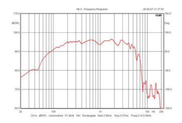
Frequency response of JA8008 from 1 metre distance, 2.8 volts input. Driver mounted on a  $32 \times 1050$  mm baffle. Response merged with nearfield response at 400 Hz.
