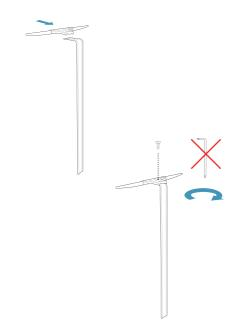
4) Place the vertical part on the screen and adjust the position.
