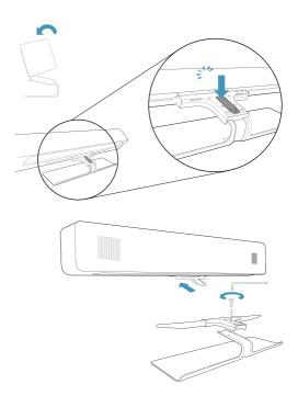
3) Attach top part to vertical part. Finger tighten the screw so that you can adjust the mounting position.
