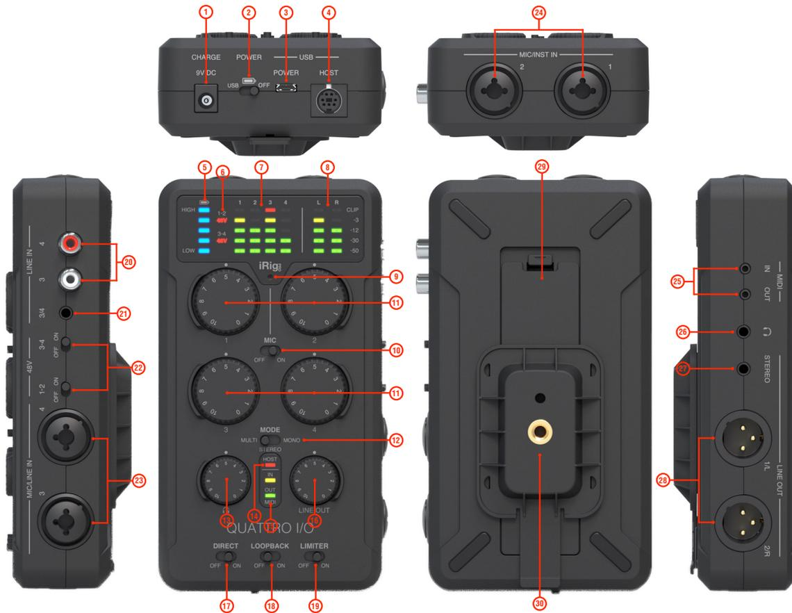
1. **External DC power input** - 2-pole barrel socket. 9V DC, 1.75A (max), positive on the external pole. When iRig Pro Quattro I/O is connected to a Lightning iOS device, using this DC In with the optional PSU (included in Deluxe version) will charge the connected iPhone or iPad.
