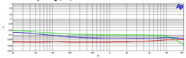
From top to bottom: 40W, 10W, 1WFrequency Response (4Ù, 8Ù and open circuit)
