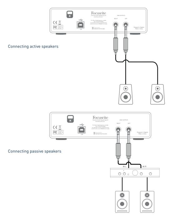
The line output connectors are 3-pole (TRS)  $\frac{1}{4}$ " (6.35 mm) jack sockets, and are electronically balanced. Typical consumer (hi-fi) amplifiers and small powered monitors will have unbalanced inputs, either on phono (RCA) sockets, or via a 3.5 mm 3-pole jack plug intended for direct connection to a computer. In either case, use a suitable connecting cable with jack plugs at one end.
