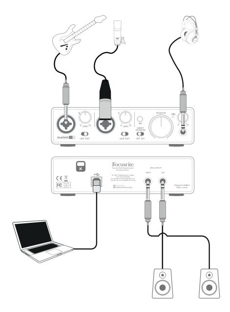
This setup illustrates the most typical configuration for recording with DAW software on your Mac or PC. In this case, you might record guitar through Input 1 and vocals through Input 2 into Ableton Live Lite, while monitoring the playback from the DAW via headphones (or speakers).
