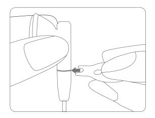
① Align the semi-circular indentation of the MMCX assist tool to the gap between the connector's male and female components.
