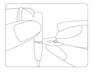
② Ensure the tool is parallel to the gap and position it towards the gap between the connector's male and female components until it is in place.
