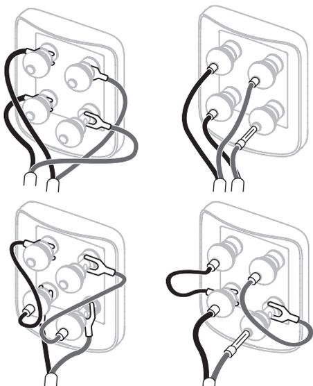
There are two pairs of terminals at the back of each speaker that enable bi-wiring (top). For conventional, single wire connection, fit the supplied link wires to join the like polarity terminals together.
