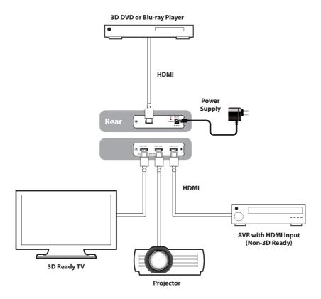
In this example, a 3D Blu-ray player is connected to the splitter allowing the HDMI output to be split to a 3D-ready LCD TV and a non 3D-ready projector. The audio output is split from the video to a non 3D-ready AV Receiver negating the need to replace the AV receiver with a newer, 3D capable model.
