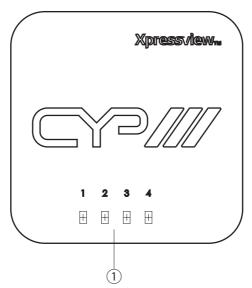
① Input LED 1~4: These LED will switch on according to user's input selection.
