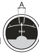
Diagram 5 Bias meter during working Note: When working normally, the pointer should stay within the A zone, still, it would move for the voltage fluctuation.
