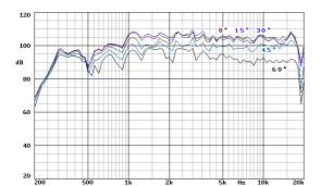
Notes: dispersion measured with two waveguides coupled to a  $90^{\rm e}$  x  $5^{\rm e}$  horn in anechoic chamber, 1w @ 2m.
