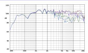
Notes: dispersion measured with two waveguides coupled to a  $90^{\circ}$  x  $5^{\circ}$  horn in anechoic chamber, 1w @ 2m.
