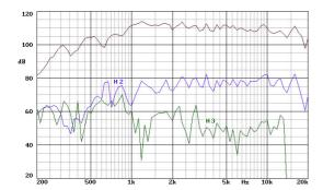
Note: on axis frequency response measured with two waveguides coupled to a 90° x 5° horn in anechoic chamber, 1w @ 1m.
