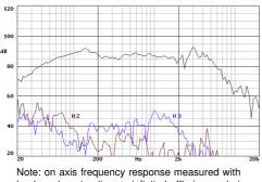
Note: on axis frequency response measured with loudspeaker standing on infinite baffle in anechoic chamber, 1w @ 1m.
