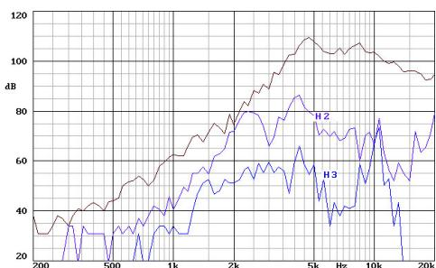
Nota: on axis frequency response measured on anechoic chamber,
