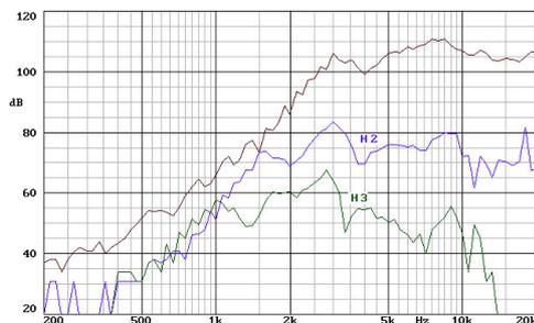
Nota: on axis frequency response measured on anechoic chamber, applying 1w@1m.
