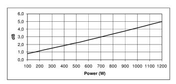
Note: These losses are calculated from a five minutes AES power test applying band limited pink noise (50-500 Hz). The loudspeaker is free-air standing.
