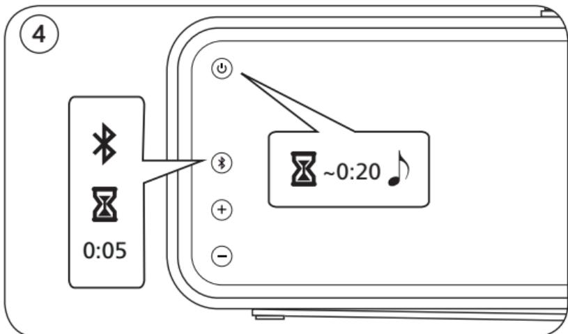
**EN** Use True Wireless to connect two speakers wirelessly. Press and hold the Bluetooth button on the first speaker for 5 seconds. Wait until a second sound prompt is heard and the power button flashes white. Then release the button. This speaker becomes the Master speaker and plays audio on the left channel. The device you are playing must be connected to the Master speaker through Bluetooth. Wait for 20 seconds until you hear a sound prompt. Then, continue to set up the second speaker.
