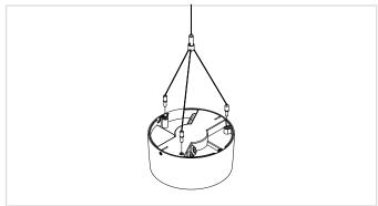
Assemble the suspension kit to the speaker through inserting the bolts of the triangular steel wire construction into the threaded bushings on the rear side of the loudspeaker.
