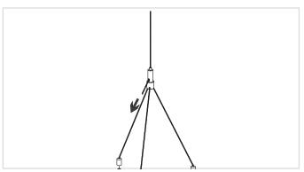
Insert the steel wire suspending from the ceiling through the connecting joint part, and pull it through until the desired height is reached. When released the speaker is instantly anchored. Verify whether the speaker is safely suspended and anchored by gently pulling it. For releasing or bringing the speaker height down, press and hold the surrounding part at the cable entry to release it.
