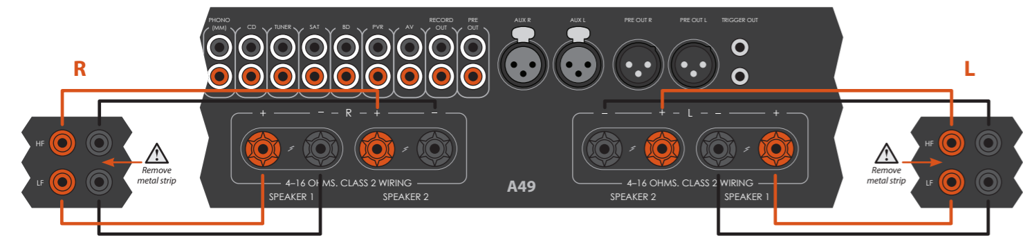
An A49 connected to two sets of speakers using bi-wiring.
