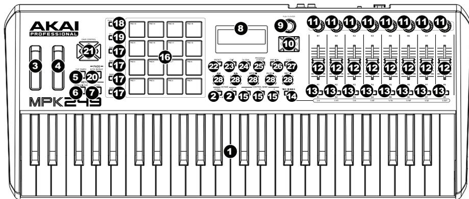
1. **Keyboard:** This 49-note keyboard is velocity-sensitive and, in conjunction with the **Octave Up/Down** buttons, can control a ten-octave range.
