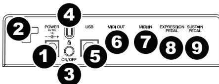
2. **Power Adapter Restraint:** You can secure a power adapter cord to this restraint to help avoid disconnecting it accidentally.
