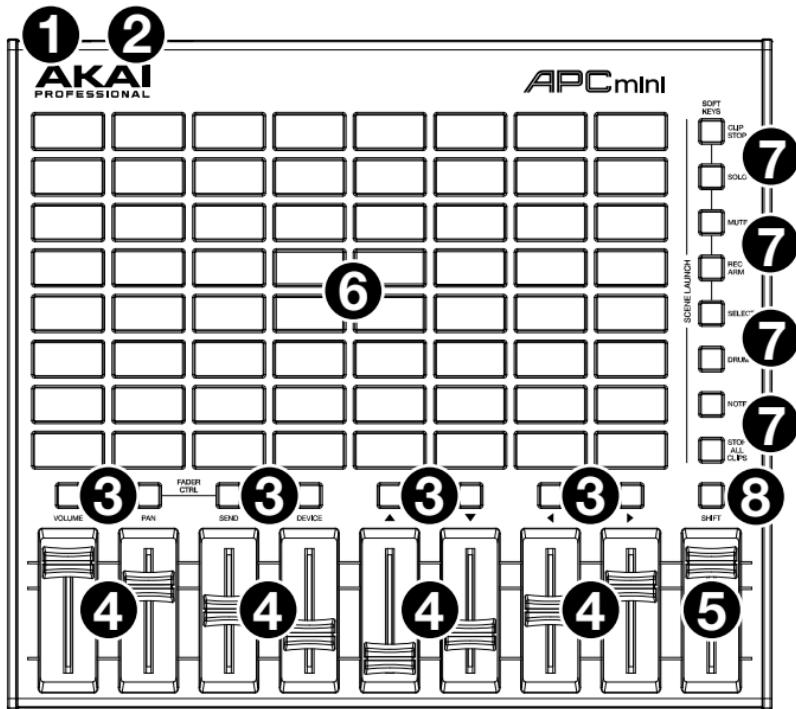
1. **USB Port:** Use a standard USB cable to connect this port to a USB port on your computer. The computer's USB port provides power to APC mini mk2. This connection is also used to send and receive MIDI data to and from your computer.
