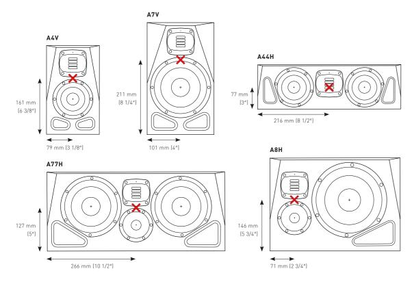
→ Ensure that the acoustical axis of your loudspeakers points towards the listening position in the horizontal plane - see diagram below.
