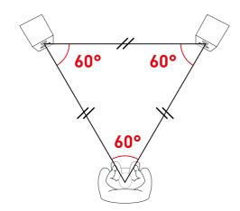
The A8H comes in two versions: left and right. Usually, they are positioned according to the naming (left picture below), however if space is limited, for example in a very narrow room, it is OK to swap the loudspeakers (right picture below). When doing this ensure that the acoustic axis is still positioned with a 60° spacing so that the stereo imaging is unaffected.
