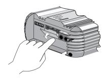
**1** - Open the transparent cover by pushing the two teeth in its lowest corners to the direction indicated by the arrows.
