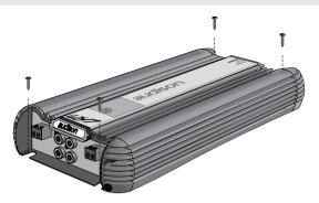
Fix the amplifier through the self-tapping screws  $(4.2 \times 16)$  given with it.
