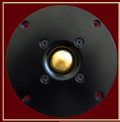
Innovation September 2005, this tweeter is equipped with a dome of 25 mm of titanium covered with gold, this in order to obtain the most rigid and light dome possible. Thanks to a specific treatment of the dome, we kept all the qualities brought by titanium (impulse response, linearity, efficiency) and removed any metal aggressiveness in the top of the spectrum. It is been driven by a powerful neodymium magnet which enables him to reach 98 dB of output.
