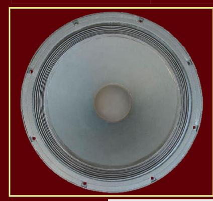
This low register driver unit of high efficiency (96 dB) offers a low register quick, deep and very pleasant to listening. Its exponential cone ensures you a broad band-width with a natural cut at 4000 Hz without accidents in run-out. Its engine made up of a ring of 3.5 kg of Alnico makes it possible to obtain the field necessary to reach a such efficiency.
