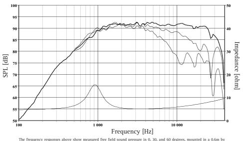
The frequency responses above show measured free field sound pressure in 0, 30, and 60 degrees, mounted in a 0.6m by 0.8m baffle. Input 2.83 V<sub>RMS</sub>, microphone distance 0.5m, normalized to SPL 1m. The impedance is measured without baffle using a 2V sine signal.
