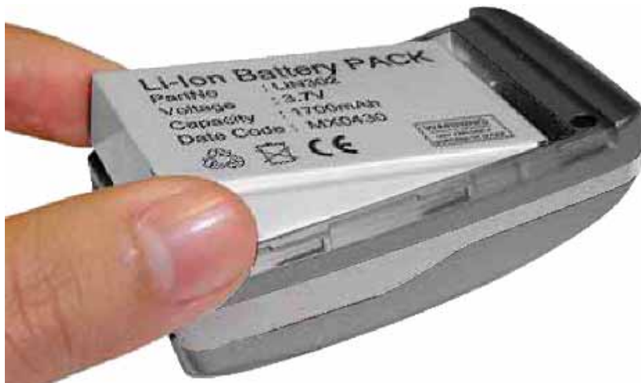
Figure 3 Put new battery into BT-339
