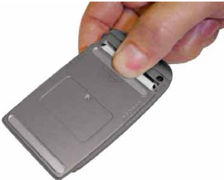
Figure 1 Open the cover of battery
