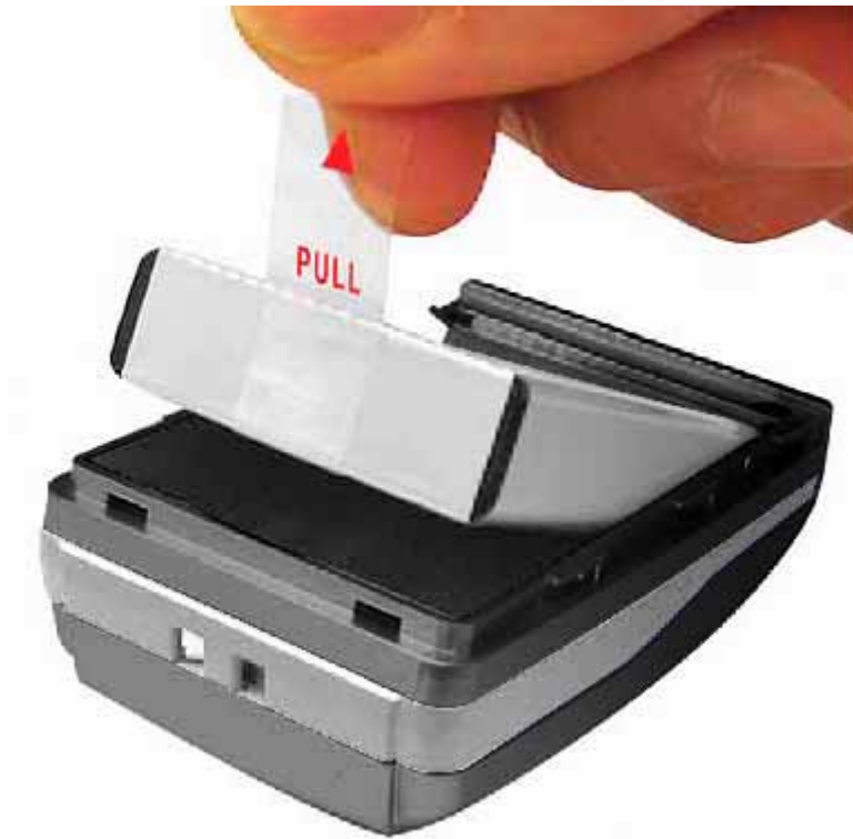
Figure 2 Take out the battery with pull tag
